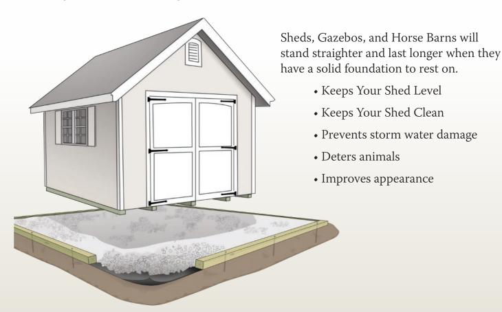
Optional 6" x 6" Pressure Treated Timber Border secured to ground with 24" steel rebar
